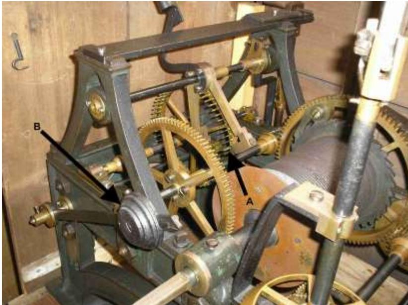
The striking train is on the right of the clock mechanism and on the quarters strikes one, two or three 'ting-tangs' on the two bells in the cupola on the top of the clock tower. On the hour the number of hours is struck on the larger bell.
